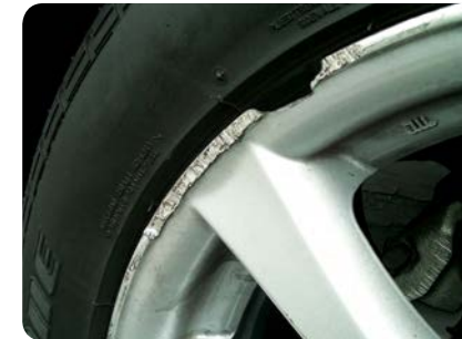
12. Damaged Alloy Wheel
